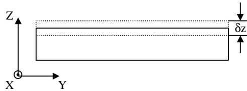
Figure 5: z-error in a layer
