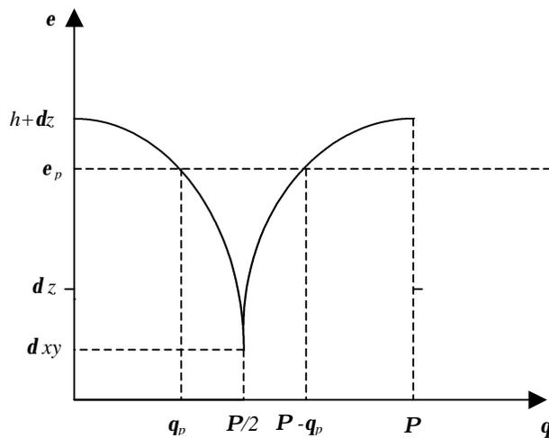
Figure 6: Effect of angle between build and face normal vectors on the flatness error
