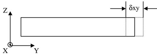
Figure 4: xy-error in a layer
