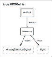
Function and flow diagram of CDS Cell.
